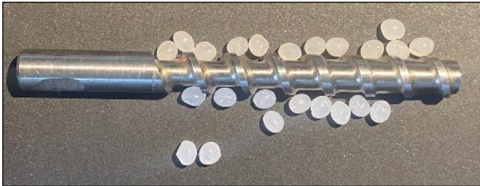
Figure 5. Image of the purchased micro compression screw with virgin PLA pellets that would typically be used for fused particle fabrication or filament manufacturing. Take note that the channel depth is significantly smaller than the diameter of the pellets.
