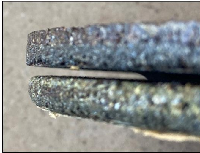
Figure 14. Comparison of a disk after 10 screws (bottom) and an unused disk (top).
