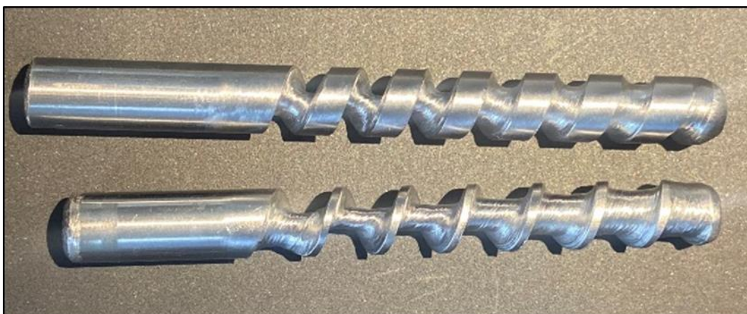
Figure 11. Comparison between a screw using a 3.175 mm thick abrasive disk (top) and a 6.35 mm thick abrasive disk (bottom).
