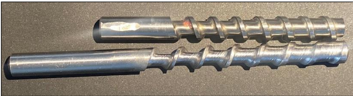
Figure 7. The top screw is the original purchased screw with a channel depth of 1.6 mm. The bottom screw was manufactured with the machine detailed in this report and has a channel depth of 2.5 mm. Both screws have an outer diameter of 8 mm.
