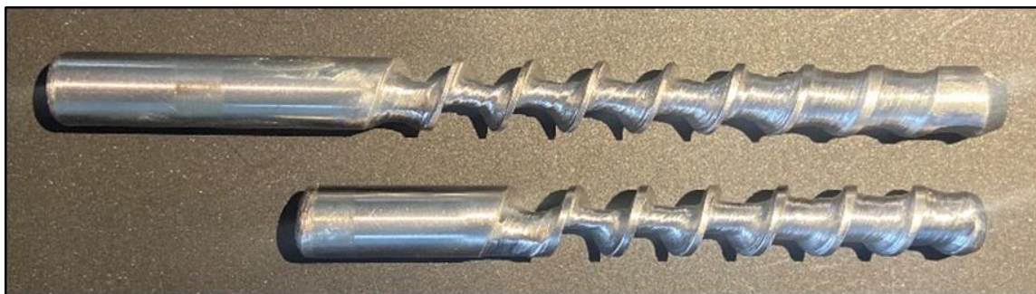
Figure 13. An example of two screws manufactured from 416 stainless steel.
