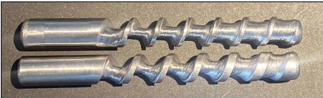
Figure 10. Comparison of two screws with a 10 mm diameter and different pitches. The top and bottom screws were manufactured using a 10 and 11.4 mm pitch, respectively.
