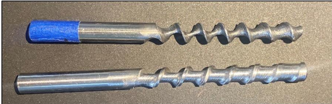
Figure 12. Comparison of a right-hand threaded screw (top) and a left-hand threaded screw (bottom).
