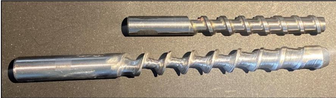
Figure 9. Comparison between the purchased screw (top) and a machined screw with an extended length (bottom).
