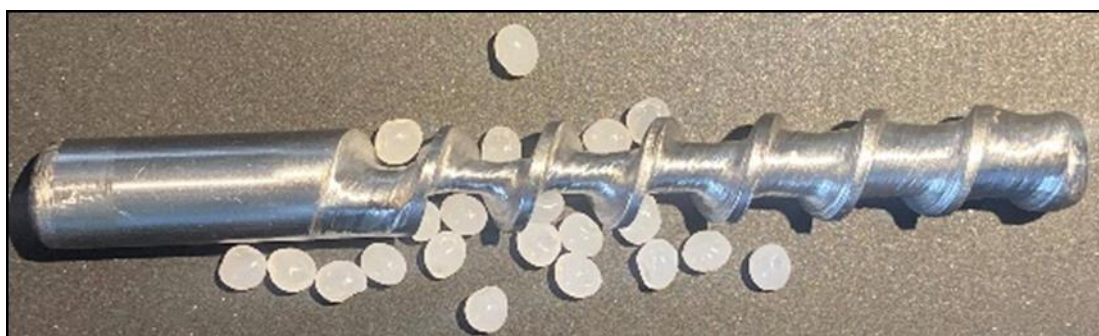
Figure 8. This screw was manufactured with a 10 mm diameter and a channel depth of 3.8 mm. Virgin PLA pellets fit nicely with these screw dimensions.
