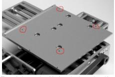
These holes need an M3 thread to be cut into. Use M3x5 screws to bolt the upper sled plate to the bed plate using these threaded holes.
